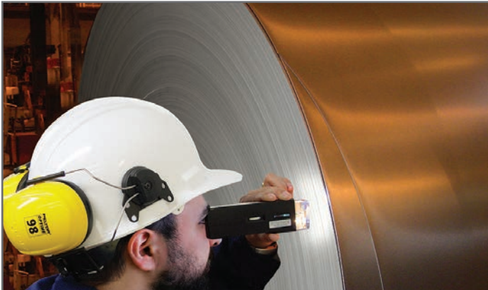
Old way of inspecting edge trim quality after the coil is completed
